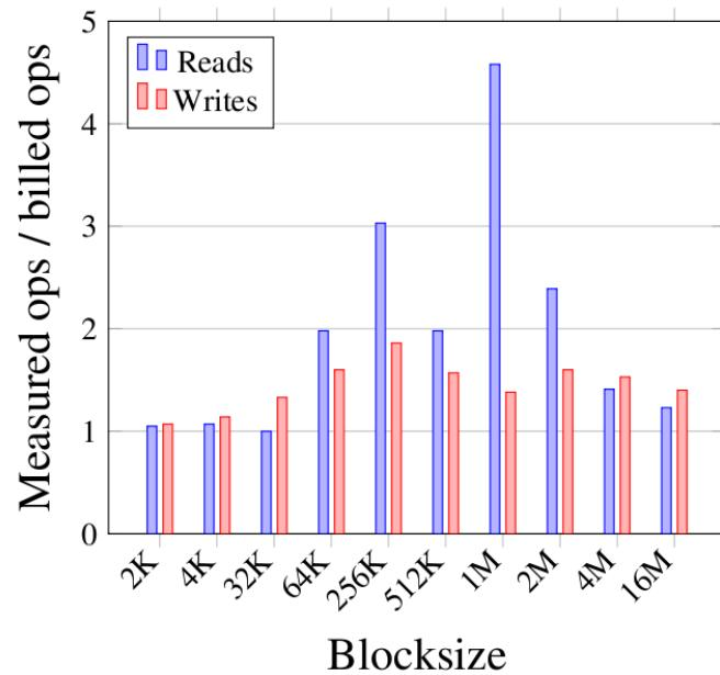
Ratio of number of storage operations measured by `/proc/diskstats` to number of operations billed by EC2.
