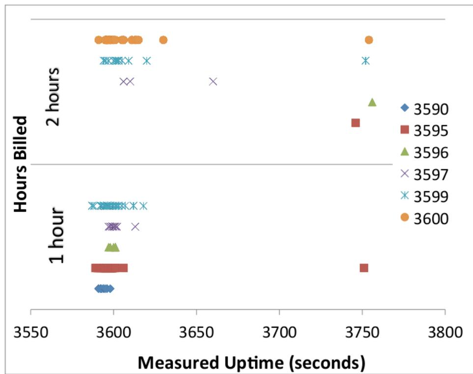
Measured uptime  $T_{down} - T_{up}$  for 272 EC2 instances run with  $3590 \leq T_{kill} - T_{launch} \leq 3600$  versus the number of hours billed.
